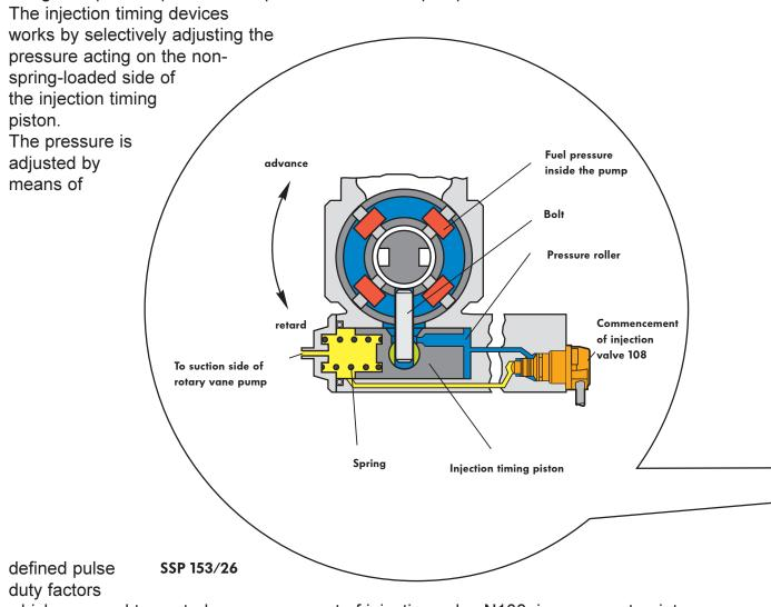
which are used to control commencement of injection valve N108, i.e. an exact point of commencement of fuel injection is assigned to each pulse duty factor. In this way it is possible to continuously regulate the point of commencement of fuel injection between max. advance and max. retard.
