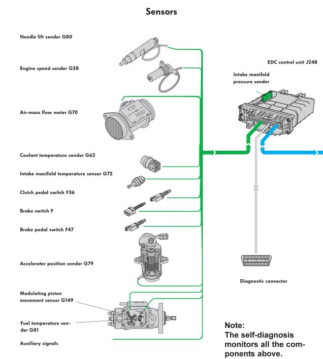
After the information supplied by the sensors has been evaluated, the control unit sends signals to the final control elements (actuators). Injection quantity, commencement of injection, charge pressure and exhaust gas recirculation are monitored and regulated in this way.
